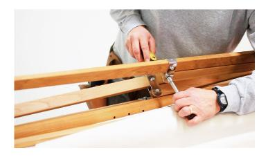
Complete the installation by attaching the end of the arm to the upper hub.
