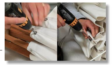
Remove the carriage bolt that holds the long and short arms together, and the elbow cover that surrounds the connection.
