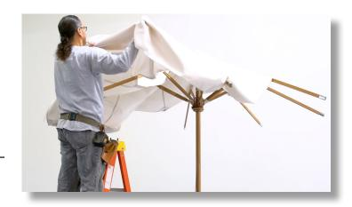
Remove the elbow covers by removing the screws that hold them in place.
