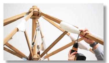
Install the new elbow covers, using the same screws and holes, if possible.
