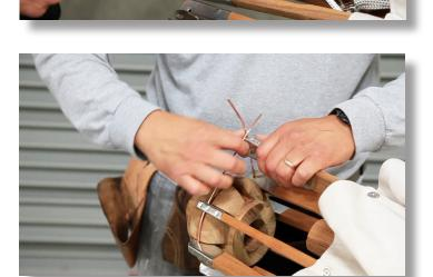
Thread the new wire through the holes in the ends of each of the arms and position the ends of the arms in the teeth of the hub.
