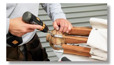
Drill three pilot holes in the new hub and attach it to the pole with the three original screws.
